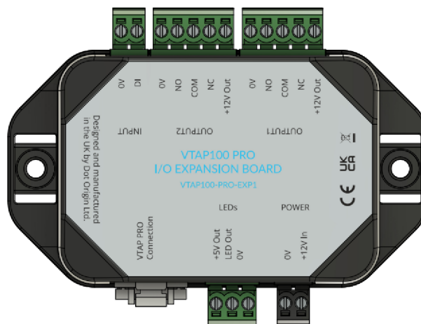
Figure 2-4 Diagram showing I/O connectors on VTAP100-PRO-EXP1
