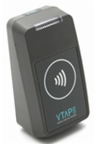
Figure 3-2 VTAP100 -CC compact case
