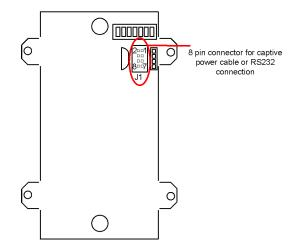
Figure 3-3 VTAP100 captive power cable or RS-232 connection v4a or v5 Hardware
